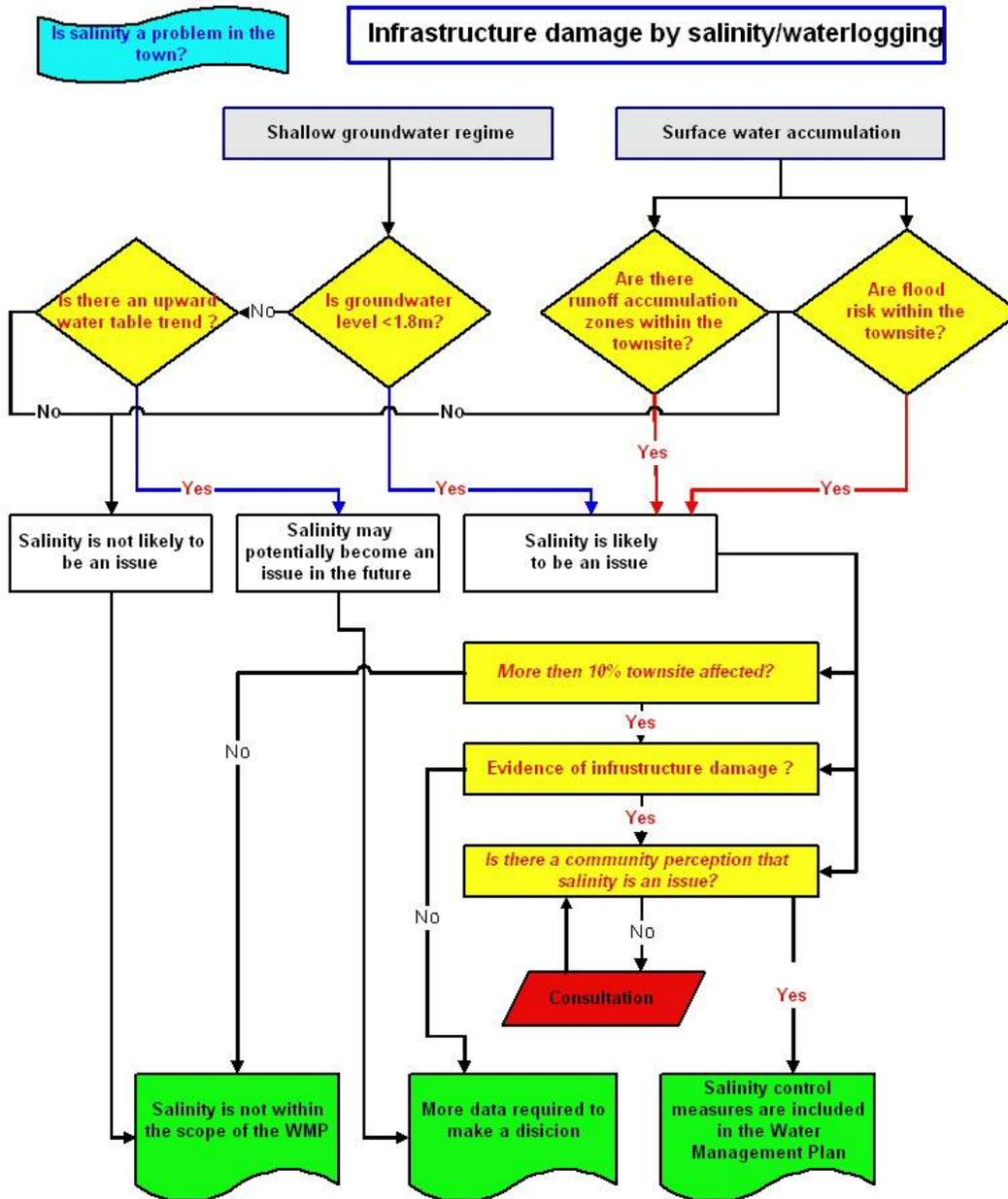
Figure I2 Infrastructure damage by waterlogging and salinity.
